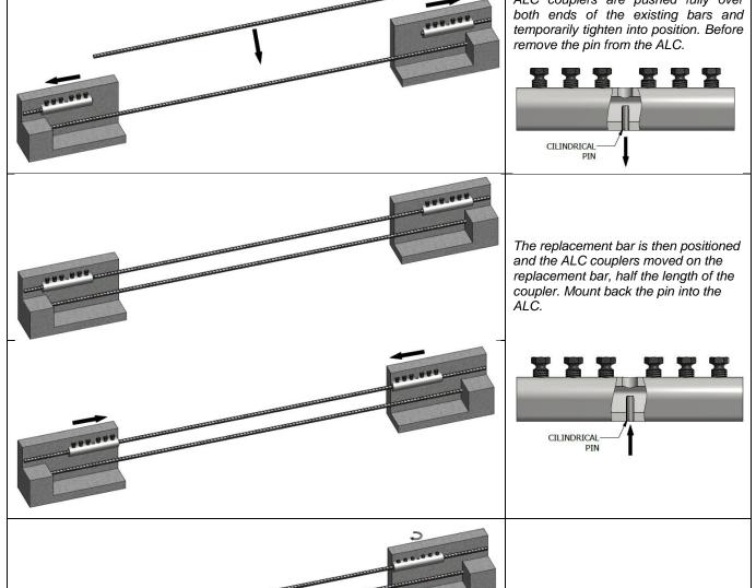
Then the breaking bolts are tightened to shear off.
