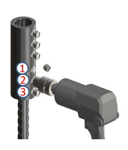
Tighten the bolts from centre to edge (from 1 to 3) with an impact wrench in several steps until the heads of the bolts shear off.
