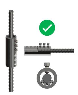
Visually control the alignment of the bar inside the coupler. It should be properly centered and rest on the centering bars. All bolts shall be in contact with the bar. For proper control please check step 3.
