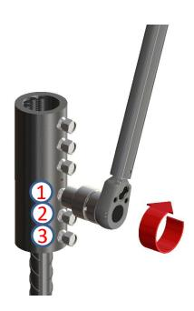
Pre-tighten the bolts with a manual wrench from centre to edge (1 to 3) of the coupler to pre-position the bar progressively and maintain its alignment inside the coupler.
