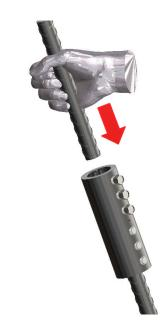
Insert the continuation bar on the other side of the Unitec coupler until it is in contact with the centre pin inside the coupler.
