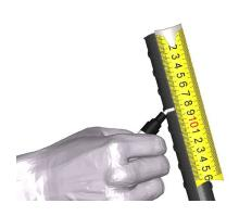
Mark the bar engagement length on each bar end, using the data provided in the table below.
