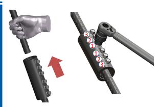
Bring the continuation bar butt-to-butt in front of it and
