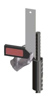
Tighten the bolts from centre to edge (from 1 to 3) with an impact wrench in several steps until the heads of the bolts shear off.
