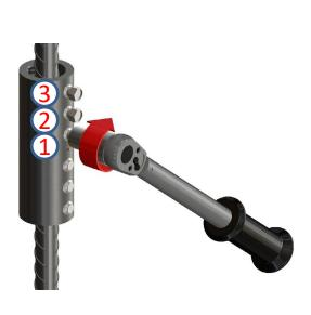
Pre-tighten the bolts with a manual wrench from centre to edge (from 1 to 3) of the coupler to pre-position the bar and maintain its alignment inside of the coupler.
